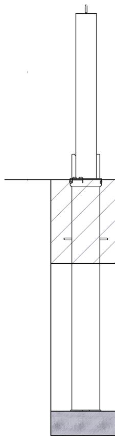
The Square RetractaPost-GL 900 is an effective means of preventing unauthorised vehicle access. When not in use, the post retracts into its integrated socket and is covered by the integral lid. The post is lockable in the raised position by rotating the post 45° and then pressing the high-security push button 7-pin security lock. The post is unlocked using the supplied key, rotated and then lowered.
