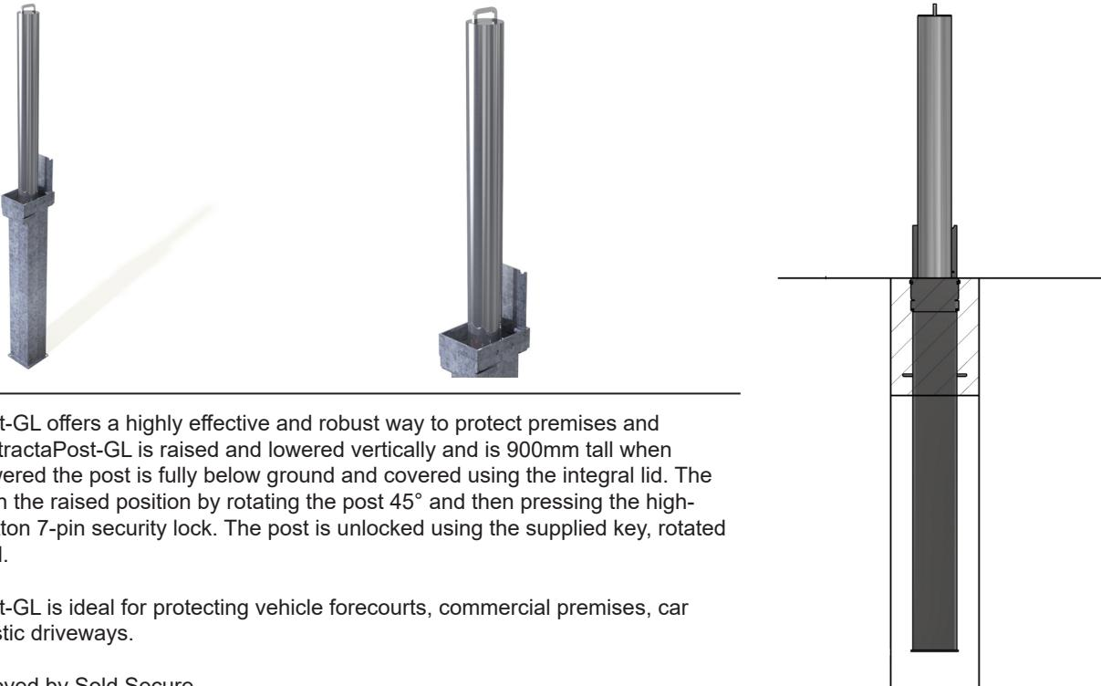
The RetractaPost-GL offers a highly effective and robust way to protect premises and vehicles. The RetractaPost-GL is raised and lowered vertically and is 900mm tall when raised. When lowered the post is fully below ground and covered using the integral lid. The post is lockable in the raised position by rotating the post 45° and then pressing the high-security push button 7-pin security lock. The post is unlocked using the supplied key, rotated and then lowered.
